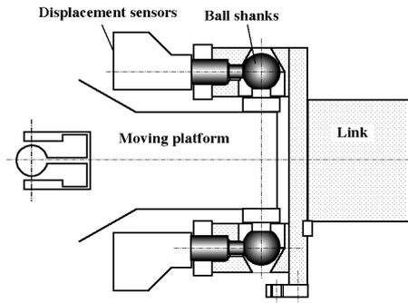
(b) Two sensors in rotational joint using two ball shanks
