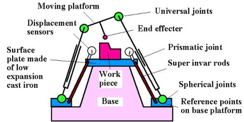
**Fig.14** Arrangement of measurement device for frame deformation in another configuration
