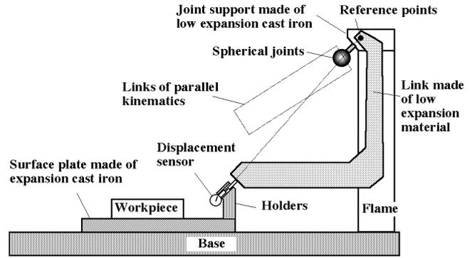
**Fig.11** Measurement device for frame deformation with curved links
