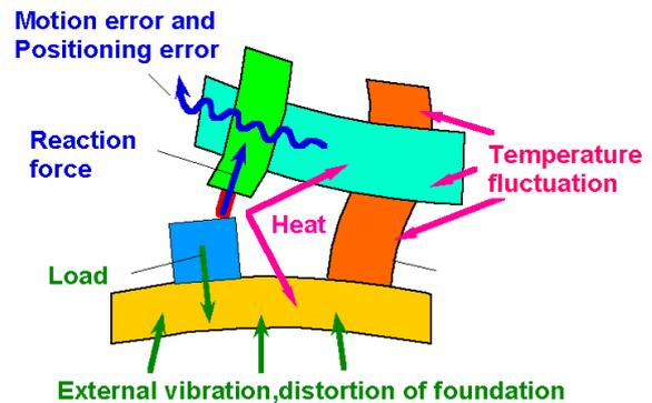
**Fig. 1** Various causes of relative positioning error between tool and workpiece for conventional machine
