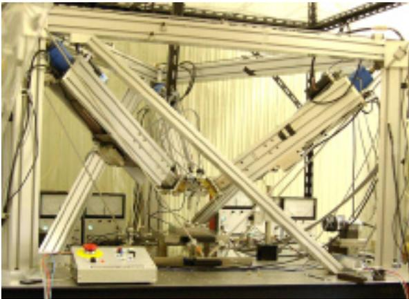
**Fig.19** Experimental CMM with compensation device for frame deformation
