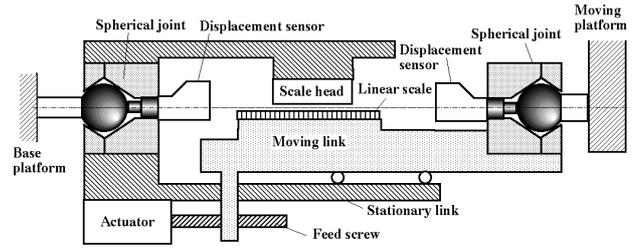
**Fig. 3** Arrangement of two displacement sensors for measuring spherical joint motion error
