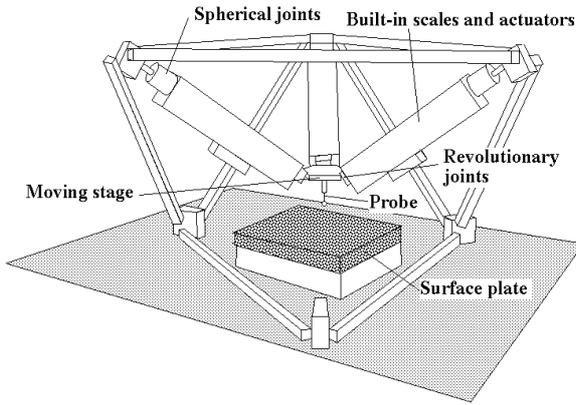
(b) Tripod type with three active prismatic joints[3][5]
