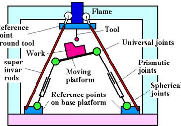
**Fig.15** Arrangement of measurement device for frame deformation in another configuration
