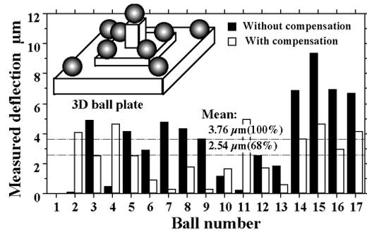
**Fig.20** Measured deflection of distances between the balls of 3D ball plate
