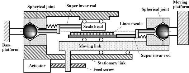
**Fig. 6** Compensation device using super invar rods connecting with reference balls and scale unit
