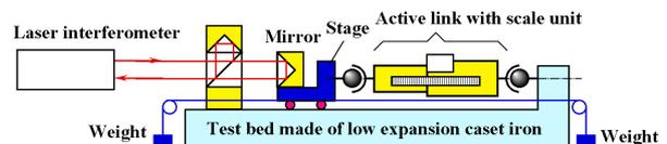
**Fig.17** Experimental setup for active link subjected to external load
