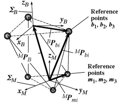
**Fig. 8** Two coordinate systems including of reference points on base platform and surface plate
