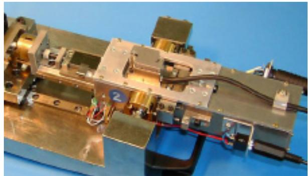
**Fig.16** Active link consisting of prismatic joint with compensation device shown in figure 6
