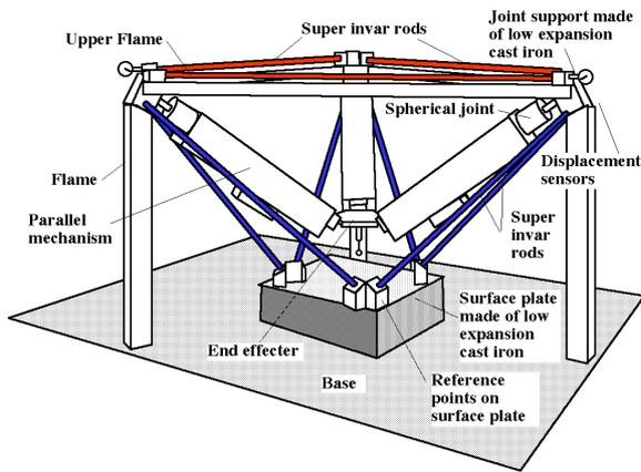
**Fig.13** Measurement device for frame deformation in 3D coordinate measuring machine
