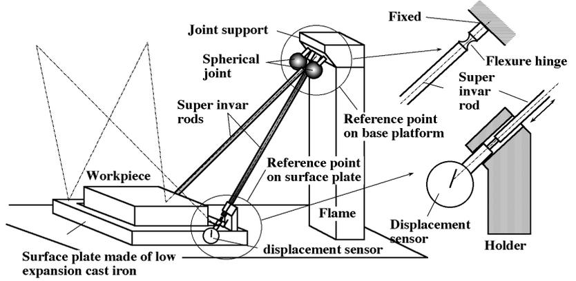
**Fig.10** Measurement device for frame deformation with 6 rods
