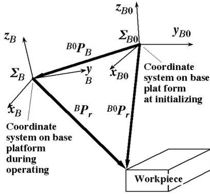
**Fig.9** Two coordinate systems at initializing and during operating
