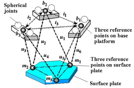
**Fig. 7** Six reference points on surface plate and base platform
