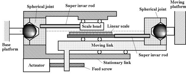
**Fig. 5** Arrangement of two super invar rods for mechanical compensation of thermal deformation of link
