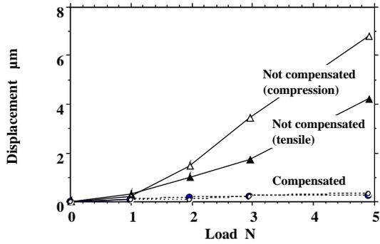
**Fig.18** Differences of measured displacements between scale unit and laser interferometer
