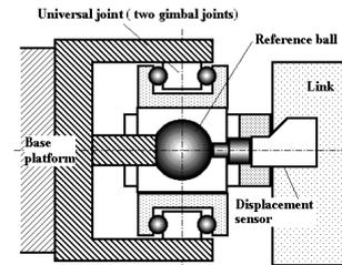
(a) Reference ball and sensor in universal joint
