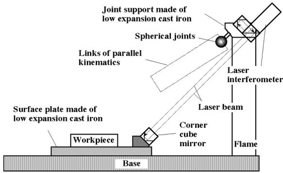
**Fig.12** Measurement device for frame deformation using laser interferometer systems
