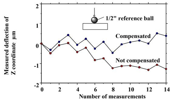
**Fig.13** Variation of the measured coordinate during measurements
