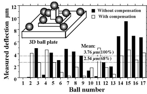
**Fig.12** Measured deflection of distances between the balls of 3D ball plate
