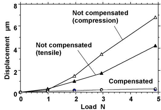
**Fig.10** Differences of measured displacements between scale unit and laser interferometer
