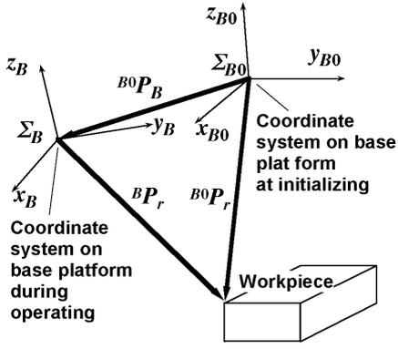
**Fig.6** Two coordinate systems at initializing and during operating
