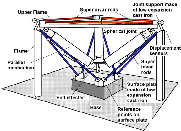
**Fig.8** Measurement device for frame deformation in 3D coordinate measuring machine
