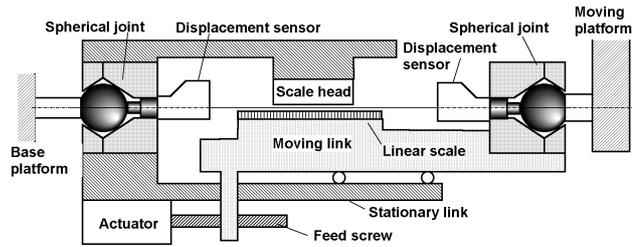
**Fig. 2** Arrangement of two displacement sensors for measuring spherical joint motion error
