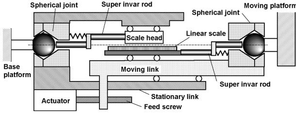
Fig. 4 Compensation device using super invar rods connecting with reference balls and scale unit
