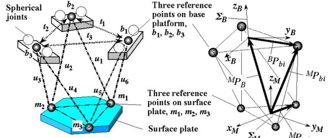
Fig. 5 Six reference points and two coordinate systems
