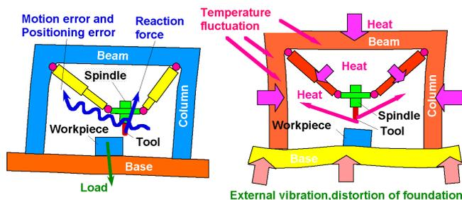
**Fig. 1** Various causes of relative positioning error between tool and workpiece for PKM
