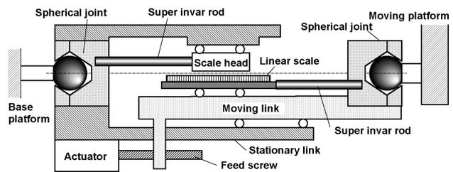
**Fig. 3** Arrangement of two super invar rods for mechanical compensation of thermal deformation of link
