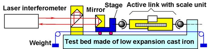
**Fig.9** Experimental setup for active link subjected to external load
