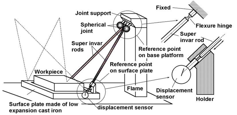
**Fig.7** Measurement device for frame deformation with 6 rods
