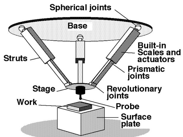
**Figure 1.** Proposed CMM based on parallel mechanism
