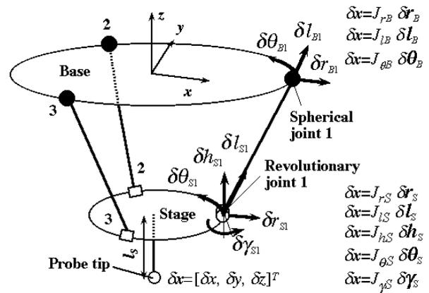
**Figure 7.** Motion errors of joints and probe tip
