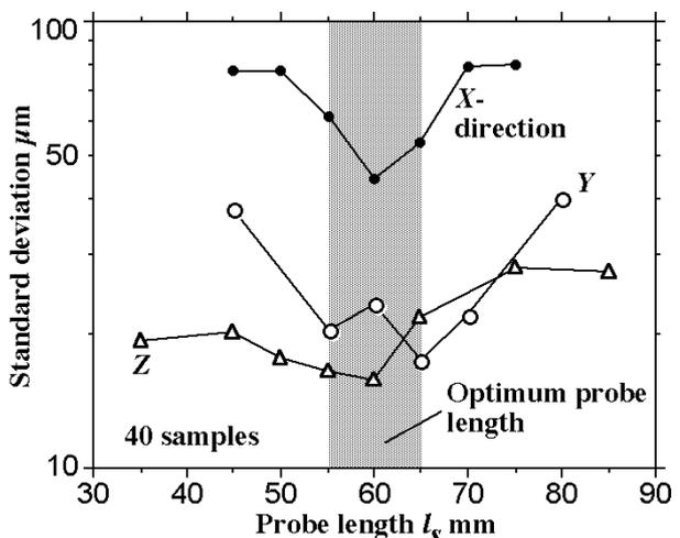
Figure 10. Influence of measuring point location on dispersion of measured value
