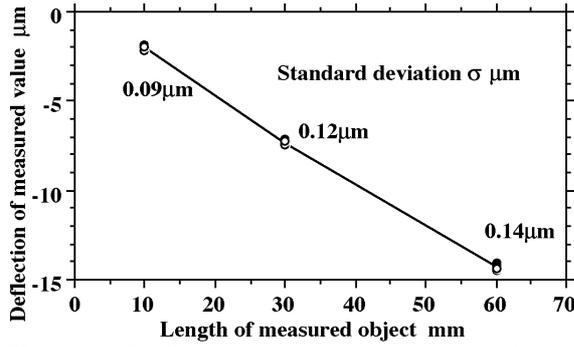
**Figure 5.** Deflection and standard deviation of measured data in Z direction before calibration
