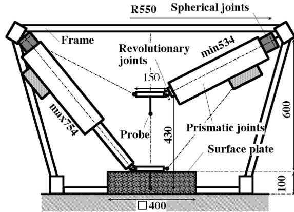
Figure 2. Scheme of experimental CMM
