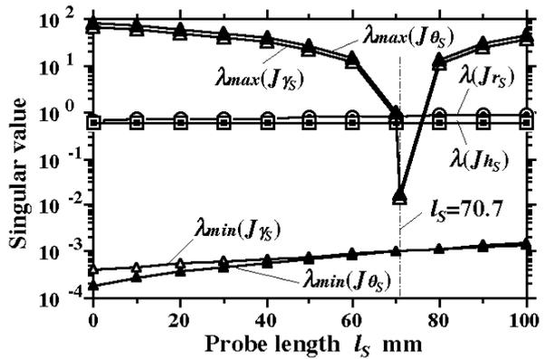
Figure 8. Influence of link layout on singular value related to stage joints
