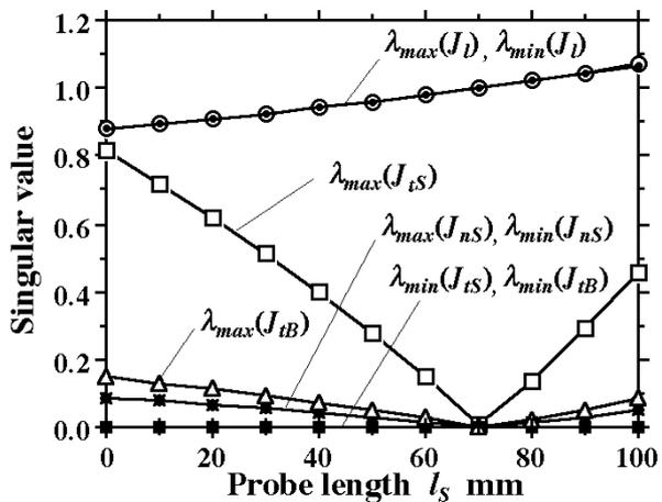
Figure 9. Effect of joint motion errors in scale direction and its orthogonal directions
